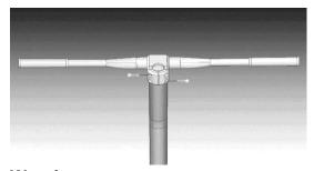
2. Only then attach the stem and the handlebar with the included screws.
