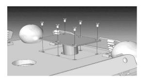
1. Insert the steering column through the hole in the board and hand tighten using the supplied Allen wrench, remove the six screws.
